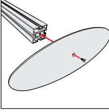
Base Plate & Extrusion Connection
